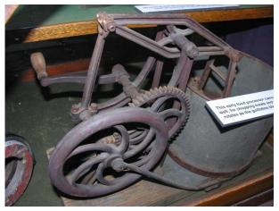
A hand-cranked food processor includes the fourth crank. The walking beam design drives a guillotine-style blade up and down with tremendous force, while the cutting board and surrounding metal bucket rotate. This device came in several sizes, none of which would be approved by OSHA today.
