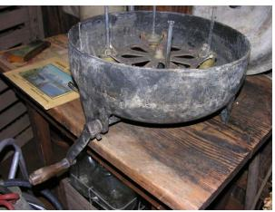
This centrifuge was used to process milk samples from different cows. It helped measure the percentage of cream in the milk, which determined the price the farmer would get. Notice the special bottles it held, with long thin necks, spun at very high speed by the fifth crank.
